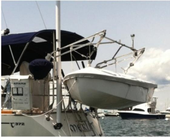
using a 1x3 piece of strapping, onto my dinghy and then put the set in my storage bin. In the spring I reverse the process once Merlin gets back on the mooring. Another option is to have your davit arms swing together once the top span bars are removed. Unfortunately with my rear radar post, this was not possible for me.
