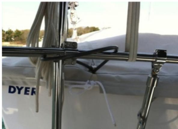
Garhauer's Davit Set includes three 1" x 8' stainless pipes and fittings to accommodate the various lengths needed for your specific rail support bars and the top davit-to-davit arm span bars.
