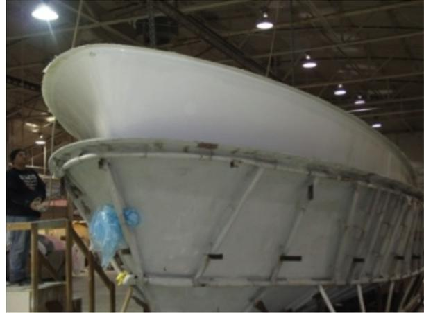
Pictured above is the hull being carefully released from the hull mold.
