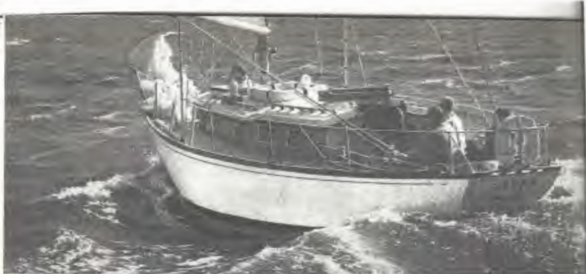
BLACK WATCH: Specifications: LOA 37', LWL 28'6", Beam 12'6", Draft w/keel 3'7", w/heel 4'6", w/boom 5'6" (boom) 8'4", S/A 50sq. 615 ft., S/A Yawl, 284 ft., CGA Rating 25.2
